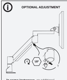
In some instances, an additional counterbalance adjustment may be needed to allow the arm's instant height adjustment function to work properly.
