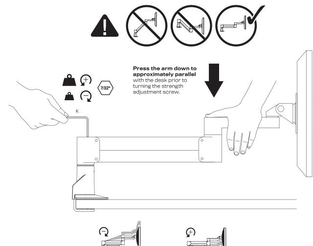
If the arm **drifts upward,** turn the adjustment screw clockwise.
