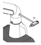
To set to a 90 degree range, use the long end of the tool to push the rotation stop switch to the side that shows a corner icon.
