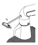
To set to a 180 degree range, use the long end of the tool to push the rotation stop switch to the side that shows a straight icon.
