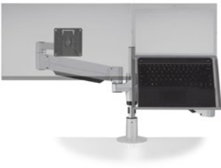
STAXX DUAL ARTICULATING w/LAPTOP HOLDER Screen Size: Up to 27" Weight Capacity: Monitor: 10 - 23 lbs. (STX-450-8510-__) 3 - 10 lbs. (STX-500-8510-__) 7 - 17 lbs. (STX-600-8510-__) 10 - 22 lbs. (STX-800-8510-__) 13 - 28 lbs. (STX-1000-8510-__) Laptop: 3 - 13.5 lbs.
