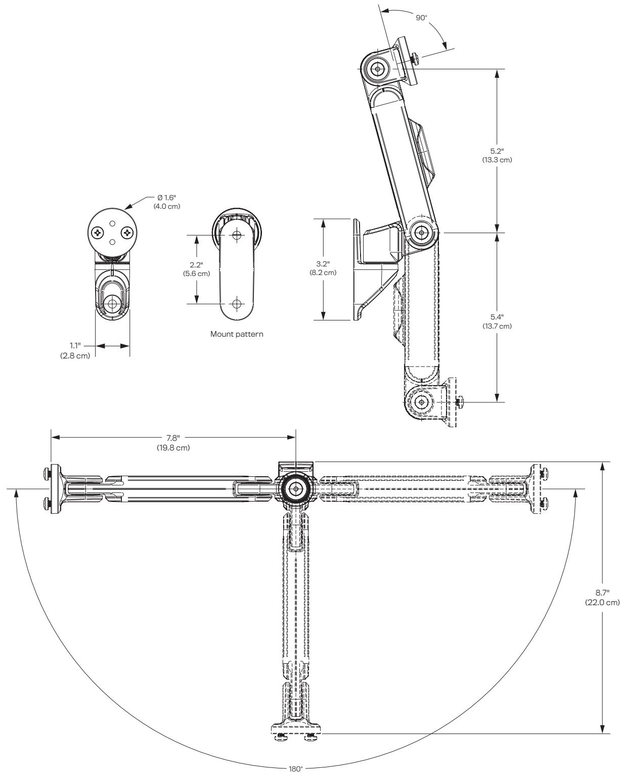
Rotation range may reduce based on device bracket installed
