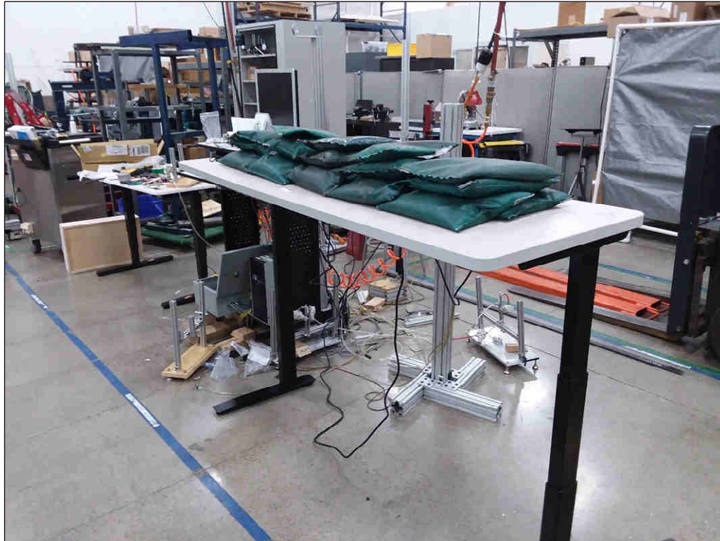
Distributed Proof Load Test
