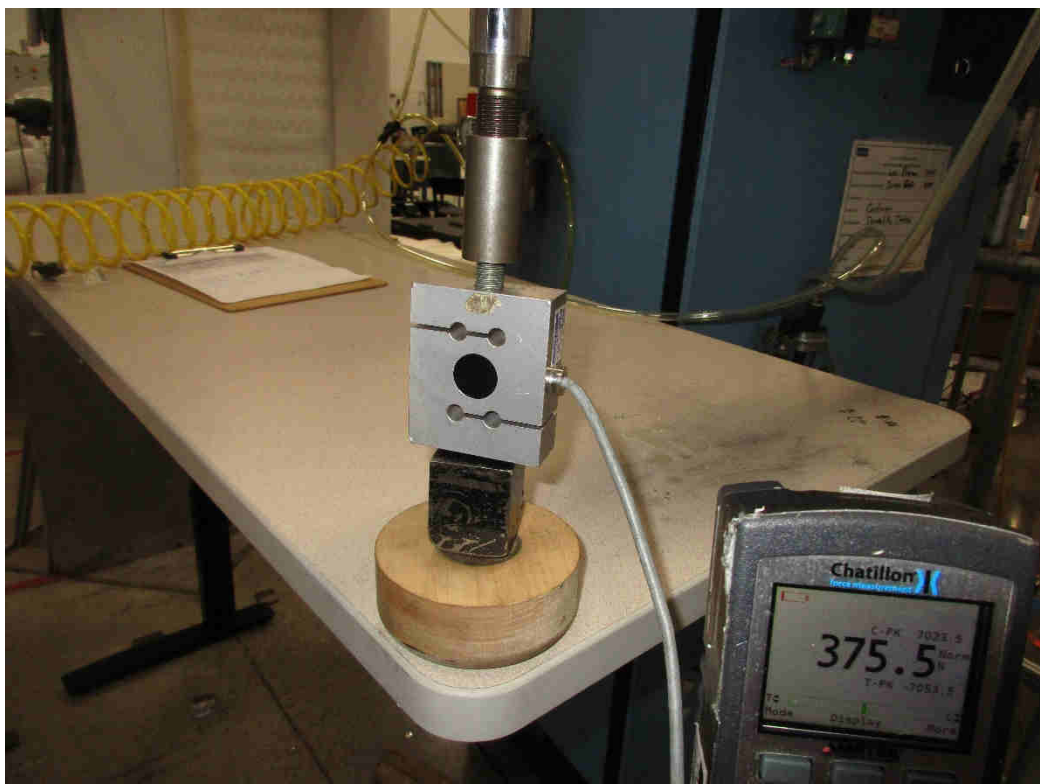
Stability Under Vertical Load
