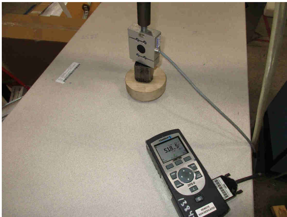
Vertical Static Load On Main Surface (1,227mm)
