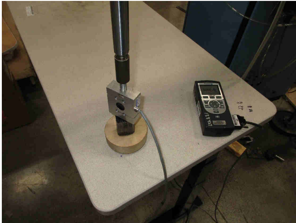
Vertical Static Load On Main Surface (950mm)
