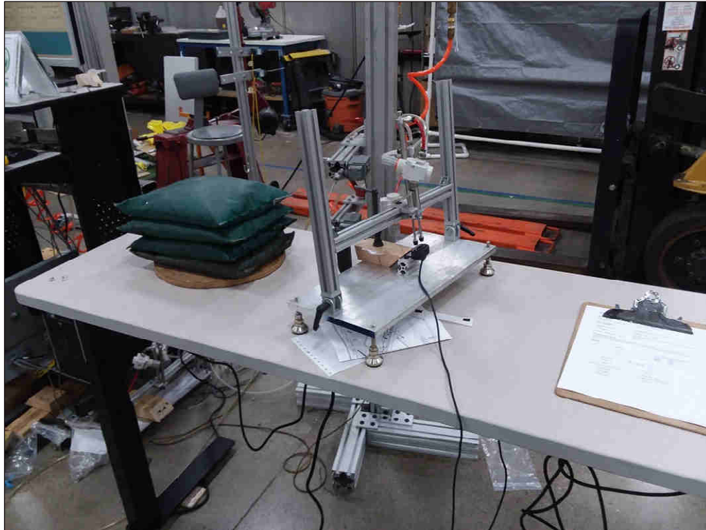
Work Surface Vertical Adjustment Test
