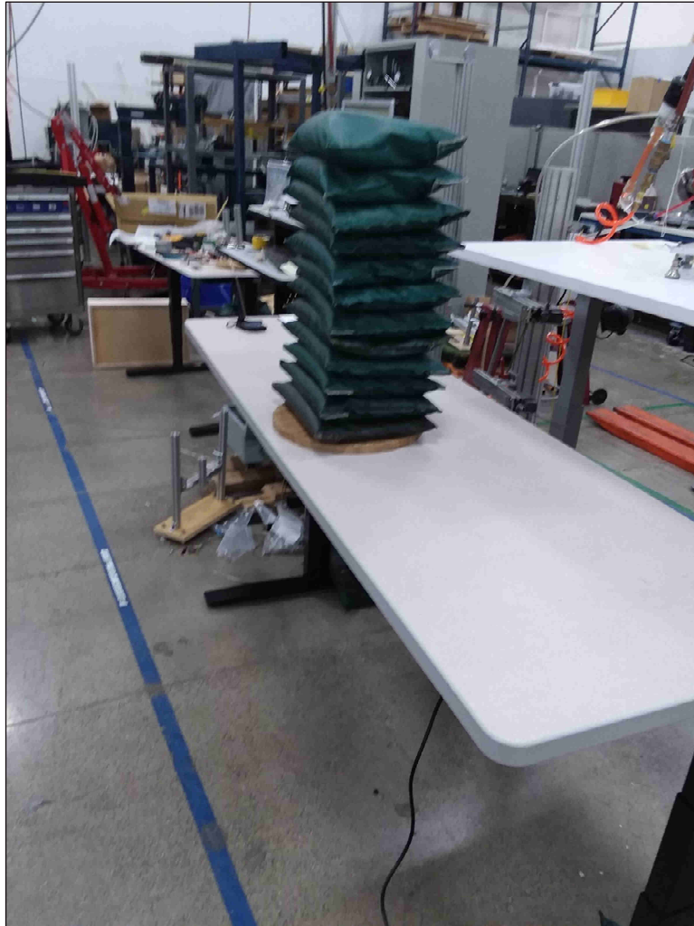
Concentrated Proof Load Test
