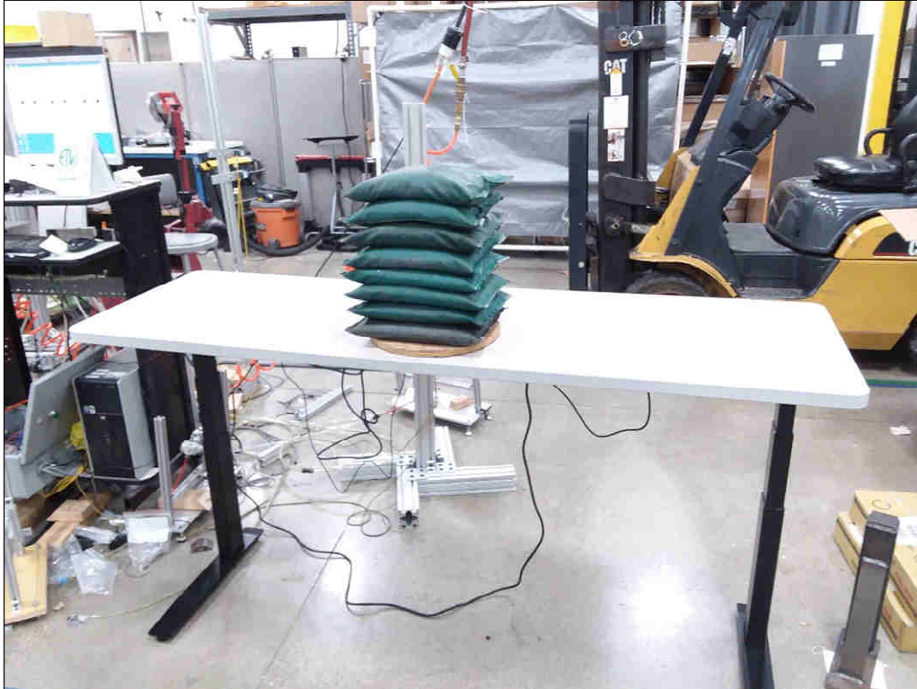
Concentrated Functional Load Test
