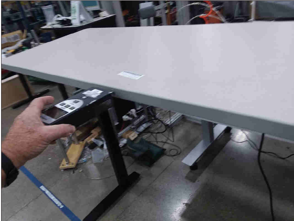
Force Stability Test for Tall Desk/Table Products
